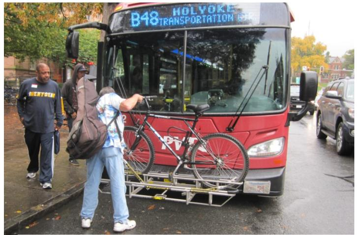
*Installation of a bicycle on a PVTA bus*
