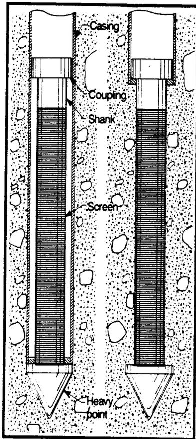
**Figure 4: Sandpoint Installed with Protective Oversized Casing.** During Driving , the casing pushed a special heavy duty drive point downward while the casing protects the screened portion of the wellpoint. The screen is exposed at the predetermined depth either by driving it with an inner casing inserted through the oversized casing or pulling back the oversized casing (Driscoll, 1986).
