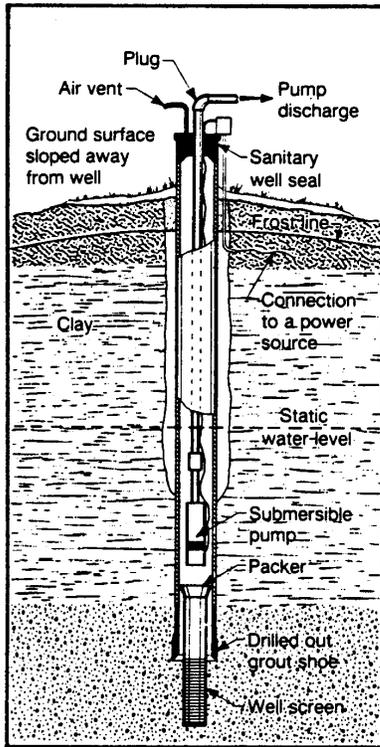
Figure 11: Properly Vented and Sealed Well (Driscoll, 1986 after U.S. EPA, 1973)
