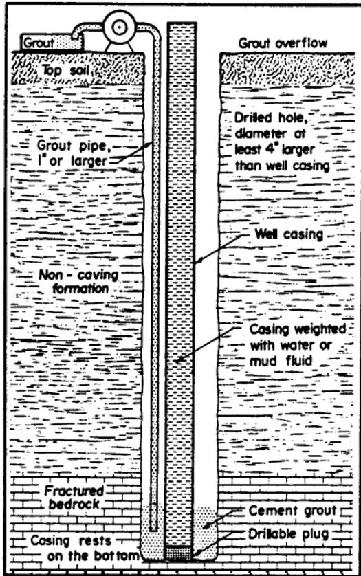
Figure 7: Grout Installation by Positive Placement Exterior Method. Grout is pumped through a pipe lowered into annular space outside the casing. (Johnson 1966)
