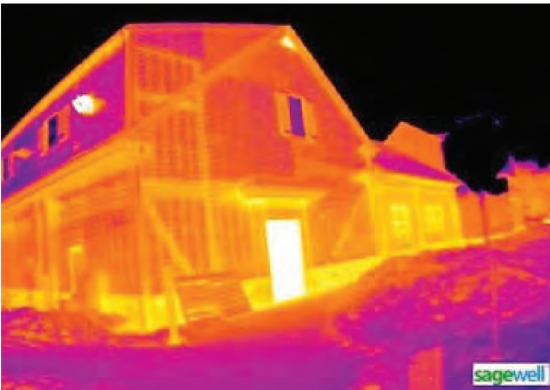
Thermal image of a house in the Pioneer Valley. Such imaging software helps auditors identify heat leaks to perform comprehensive energy retrofits.
