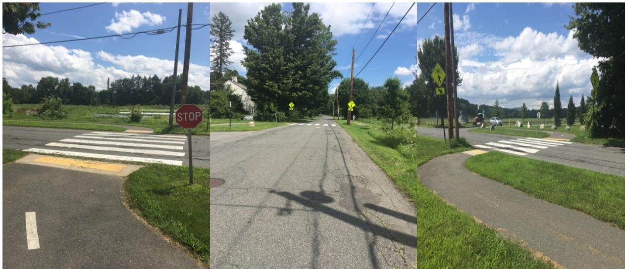
**Remarks:** It is recommended that a 'Stop sign and stop line be installed for the northbound approach of the shared use path.
