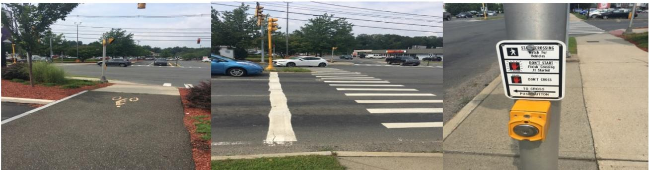
**Remarks:** The crossing is located at a four way intersection of King Street with the Shopping Center. The shared use path signs and advance warning signs along the roadway are missing. It is recommended that a median be considered for the King Street crosswalk to allow for pedestrian refuge area while crossing multiple lanes of traffic.
