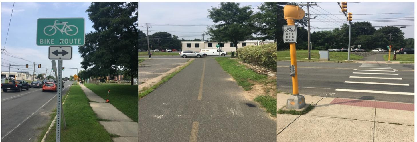
**Remarks:** The crossing is located in commercial area with a high volume of traffic and shared use path users. The shared use path connects to the sidewalks in the vicinity of the shopping center. The signal allocates approximately 20 seconds of walk time to cross King Street. Proposed King Street Reconstruction project is currently at 75% design stage which proposes narrowing down of King Street south of the crossing to accommodate bike lanes.
